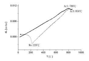
Fig. 4. Phase transformation point of the newly developed steel examined by dilatometer.
