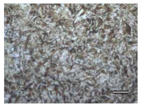
**Fig.8.** OM morphology for 860 -15min. austenitizing and oil quenching specimen.
