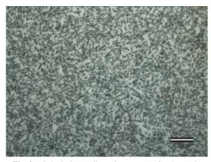
Fig. 2. Spherical annealing microstructure for the newly developed steel.
