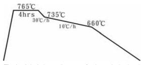
Fig. 1. Spherical annealing patent for the newly developed steel.
