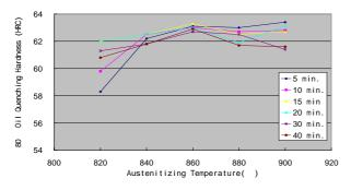
**Fig. 7.** Hardness curves of oil quenching specimens for the newly developed steel.
