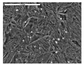
**Fig. 9.** SEM morphology for 860 -15min. austenitizing and oil quenching specimen.
