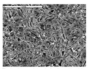
**Fig. 11.** SEM morphology for for oil quenching (860 -15min.) and tempering (170 -2hrs) specimen.
