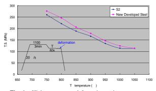
Fig. 6. High temperature deformation resistance curves for the newly developed steel and S2 steel.
